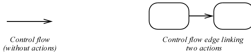
Figure 244 - Control flow notation
