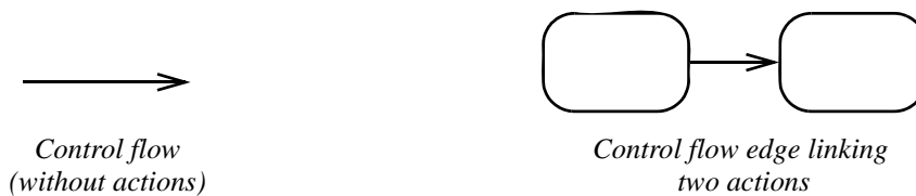
Figure 12.70 - Control flow notation
