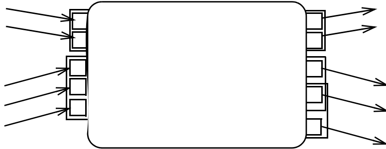
Figure 12.117 - Alternative input/outputs using parameter sets notation
