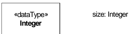
Figure 11.19 - Notation of data type: to the left is an icon denoting a data type and to the right is a reference to a data type that is used in an attribute.
